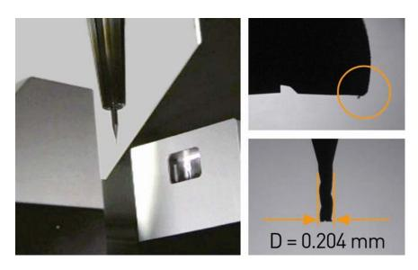
3. An example application: a reflective mirror insert - machined on a MIKRON HSM 400U LP Precision
